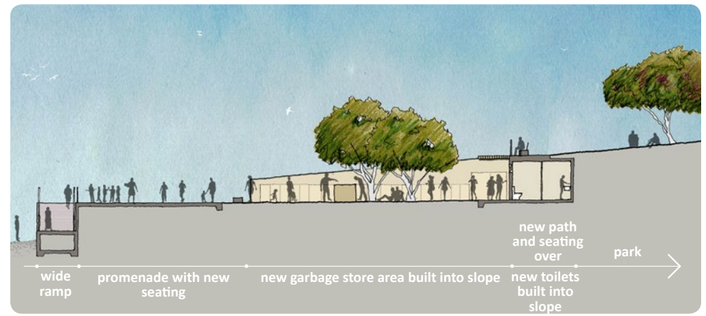
Figure 8.16 Concept section through Biddigal Park showing new toilets and garbage store area recessed into the slope
